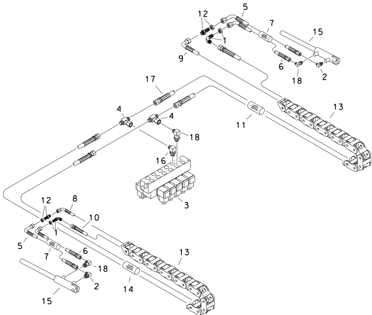
**PIPE GRIPPER HYDRAULICS**
